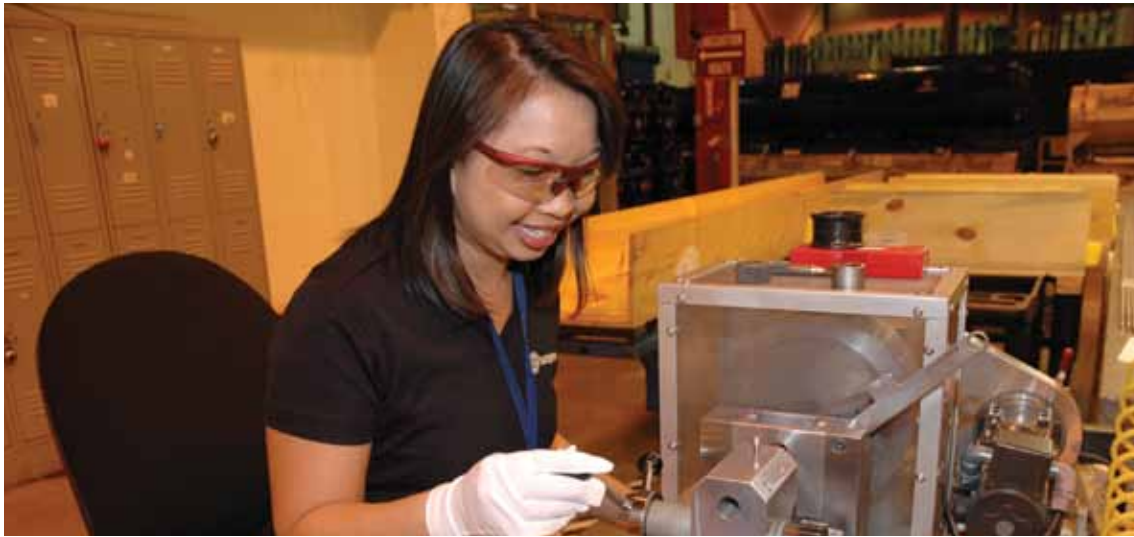
WOMEN IN NUCLEAR ENERGY. Amy Buu at a station that inspects guide thimble tubes, a component of a fuel assembly.
